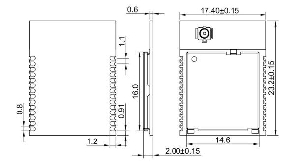
Important:Unit: mmTolerance: +/- 0.1, defaultRecommend solder pad size:1.8\*0.8mm, solder pad is suggested to extend 0.7mmdistance.
