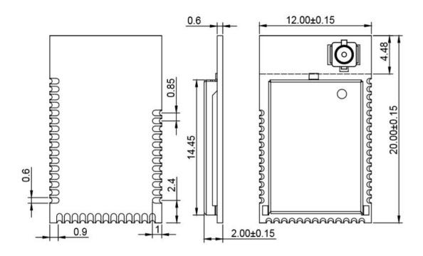
**Important:** Unit: mm Tolerance: +/- 0.1, default Recommend solder pad size: 1.7\*0.6mm, solder pad is suggested to extend 0.8mm distance.
