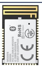
The MS50SFB is a compact and small size Bluetooth 5.1 module with ultra-low power consumption and optional antenna types; The module has the large number of GPIOs and excellent RF performance.
