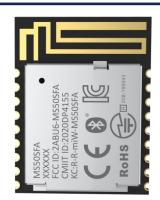
MS50SFA is a compact ( $15.8 \times 12.0 \times 2.0 \text{ mm}$ ), highly flexible, ultra-low power wireless BLE 5.0 Module based on nRF52810 SoCs; Its powerful 32-bit ARM CortexTM M4 CPU, a 192KB Flash memory, a 24KB RAM and integrating a 2.4 GHz transceiver can offer the perfect solution for Bluetooth connectivity.
