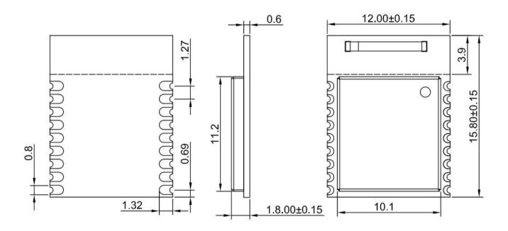
**Important:** Unit: mm Tolerance: +/- 0.1, default Recommend solder pad size: 1.8\*0.8mm, solder pad is suggested to extend 0.5mm distance.
