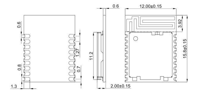
Important:Unit: mmTolerance: +/- 0.1, defaultRecommend solder pad size:1.8\*0.8mm, solder pad is suggested to extend 0.5mm
