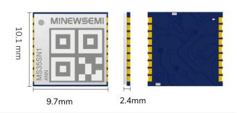
MS35SN1 is a multi-galaxy, concurrent, simultaneous multi-constellation positioning and L1+L5 positioning GNSS module. Built-in MTK advanced process GNSS Soc chip, integrated ARM Cortex-M4 FPU and MPU with a main frequency of up to 530MHz. The module supports GPS, BDS, GLONASS, GALILEO and QZSS with excellent positioning performance while maintaining low power consumption.
